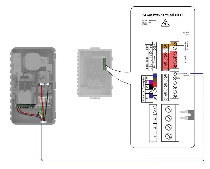
Risk of electrocution and equipment damage! Do not install CTs when current is flowing in the sensed circuit. Always install CT wires in the terminal blocks before energizing the sensed circuit.
