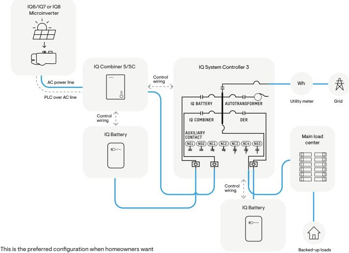
complete energy independence. This is the most powerful configuration available that ensures a home can remain powered even if the utility grid shuts down. Depending on the size of the solar and battery installed, the home can withstand grid outages for days at a stretch.
