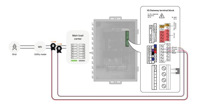
Risk of electrocution and equipment damage! Do not install CTs when current is flowing in the sensed circuit. Always install CT wires in the terminal blocks before energizing the sensed circuit.
