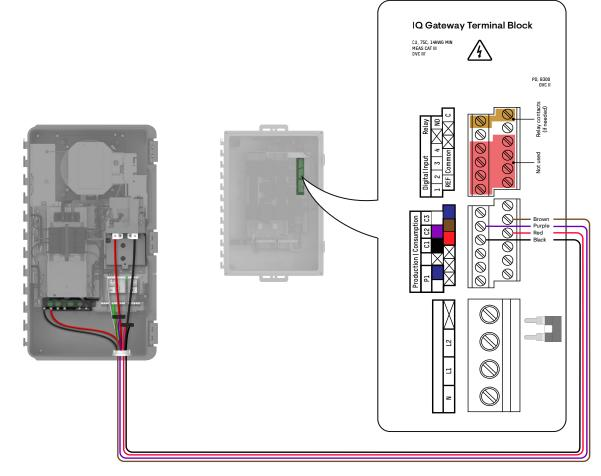
Risk of electrocution and equipment damage! Do not install CTs when current is flowing in the sensed circuit. Always install CT wires in the terminal blocks before energizing the sensed circuit.
