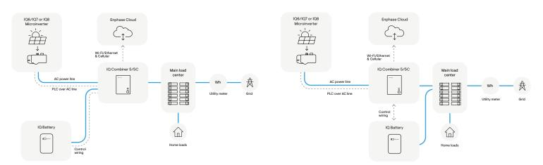
This is the preferred configuration when homeowners want to minimize their utility bill, reduce their carbon footprint, and have the option to save the excess power generated by their solar system for consumption in non-sunlight hours. A site can store the energy the solar system makes and use it anytime, day or night, rain or shine.
