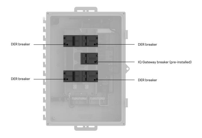
**NOTE:** On grid forming sites, IQ Batteries must land in the IQ System Controller 3/3G and must not be installed in the IQ Combiner.
