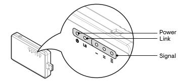
The following tables list the LED indicator status. The LEDs may be difficult to see if you view them from an angle. View the LEDs from the front for a clear view of the LED color.
