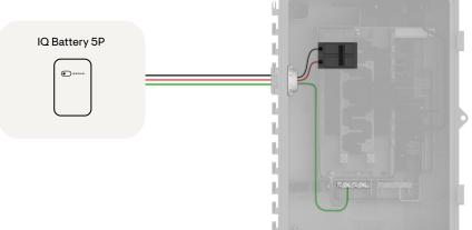
**NOTE:** Do not pass conductors from IQ Battery 5P branch circuits through the Production CT. This will distort production readings.
