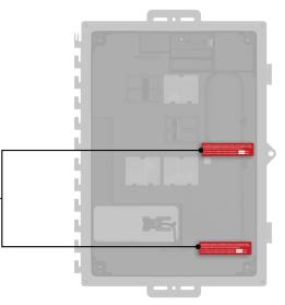
7. The IQ Combiner 5/5C accessory kit also includes an EPC label for current transformers (CTs). Use these to apply on the appropriate current transformer that enables the EPC functionality.
