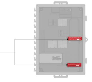
5. For sites with Aggregate export power limiting (PEL) enabled, indicate, with a label, the maximum current setting for backfeed from the solar system to the utility service that is controlled by EPC.
