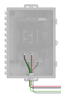
For grid-forming systems, connect the L1, L2 output from the mains lugs on the IQ Combiner to the PV lugs on the IQ System Controller 3/3G.
