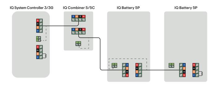
CTRL cable - - - Drain wire L<sub>w</sub> Termination resistor
