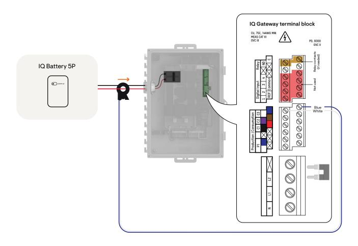
Risk of electrocution and equipment damage! Do not install CTs when current is flowing in the sensed circuit. Always install CT wires in the terminal blocks before energizing the sensed circuit.
