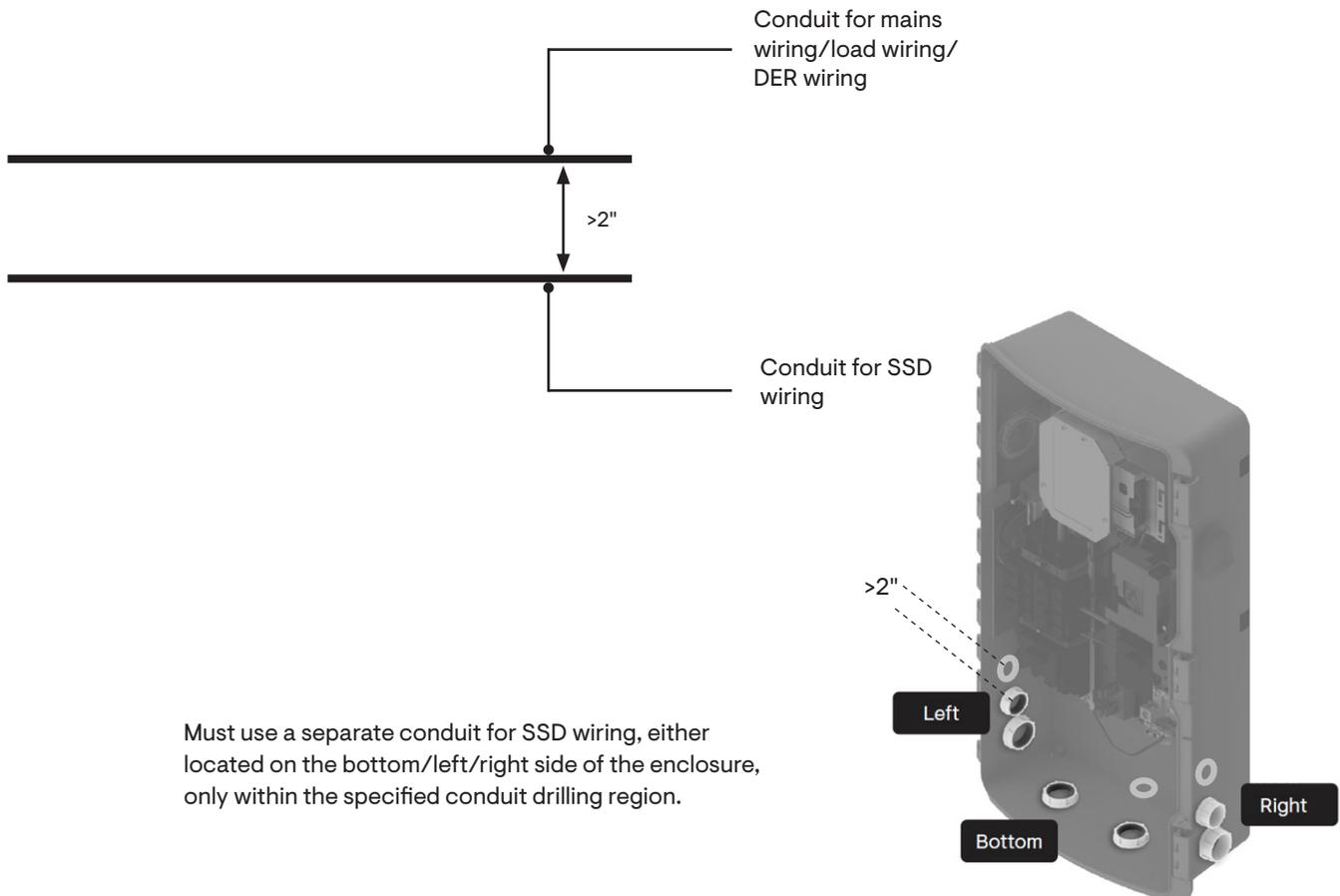
**Warning:** To prevent water ingress, do not use the top conduit entry on System Shutdown Switch.
