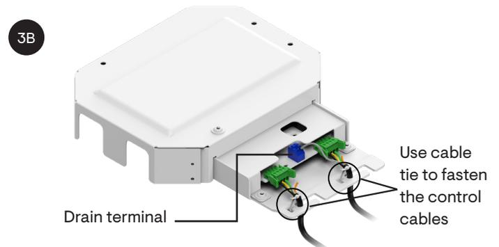
**Scenario B:** IQ System Controller is not the terminal node for the wired control network. Use a control cable of length 40 inches + conduit length on each side.
