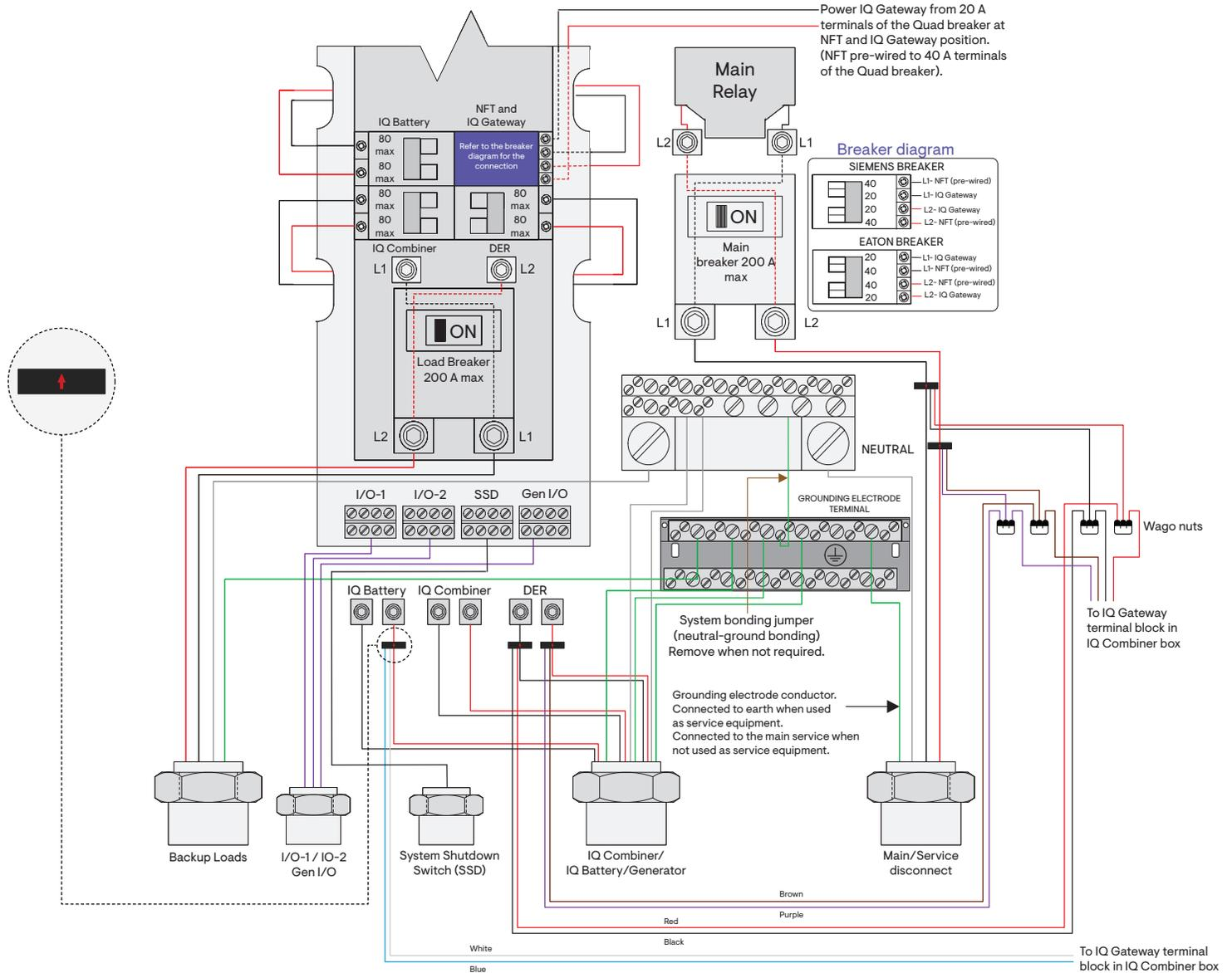
Battery CT shall be placed on the L2 wire from the IQ Battery port.
