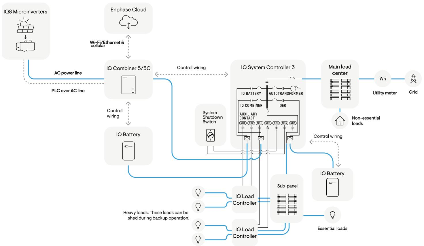
**Note:** The System Shutdown Switch is not used for IQ6, IQ7, and M Series systems. Refer to the [System Shutdown wiring](#) section for details.
