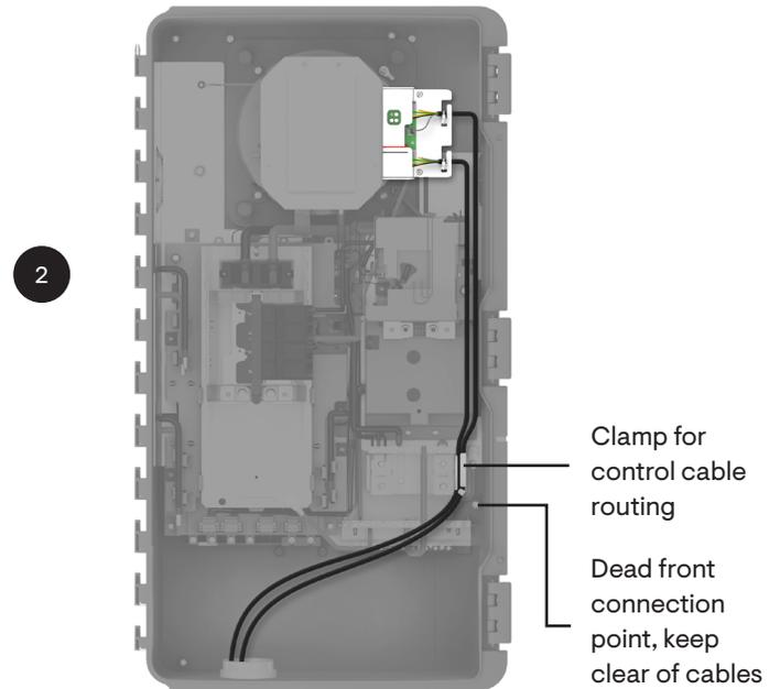
Control cable routing inside IQ System Controller. Do not use side conduits for control cable routing.
