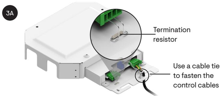
**Scenario A:** IQ System Controller is the terminal node for the wired control network. Use control cable of length 40 inches + conduit length and use termination resistor provided with Lit Kit.
