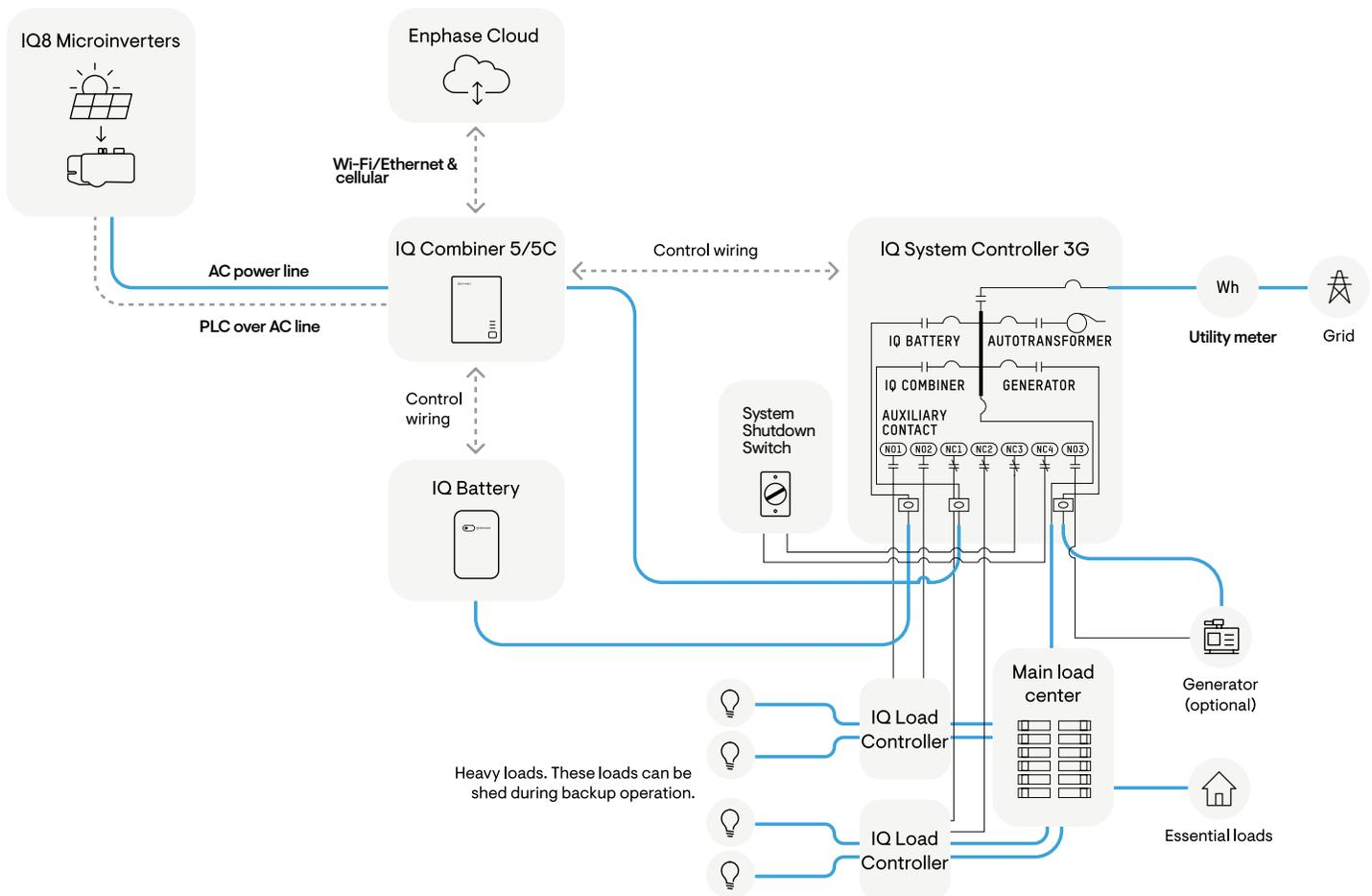
**Note:** The System Shutdown Switch is not used for IQ6, IQ7, and M Series systems. Refer to the [System Shutdown wiring section](#) for details.
