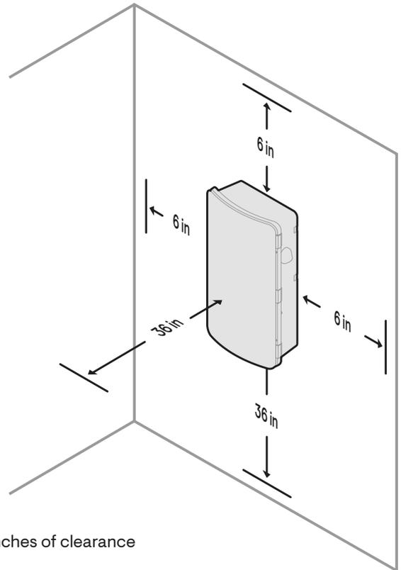
**NOTE:** If installed indoors, the IQ System Controller 3/3G requires at least six inches of clearance from the floor. Follow all local standards and regulations related to mounting.
