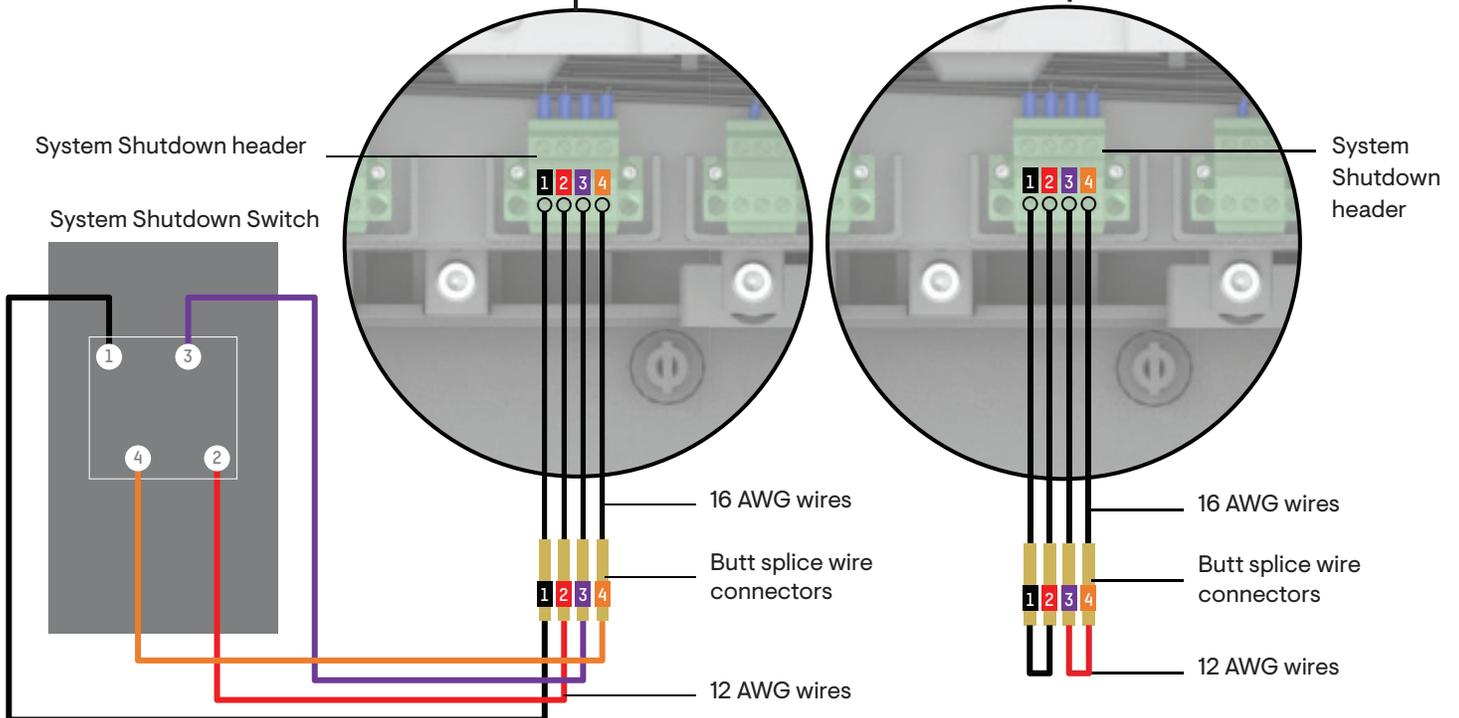
✓ **NOTE:** Control lines to headers support 28 AWG and 16 AWG wire gauges.
