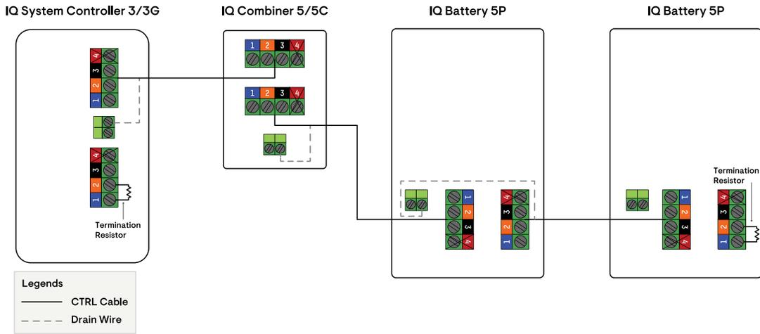
✓ **NOTE:** Total length of CTRL wiring across the system cannot exceed 250 feet to ensure the system operates as per specifications.
