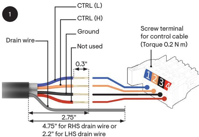
Control cable to be stripped to recommended dimensions and connected to the header.
