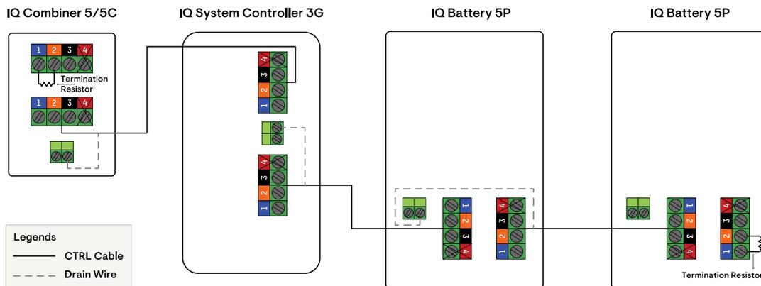
✓ **NOTE:** Total length of CTRL wiring across the system cannot exceed 250 feet to ensure the system operates as per specifications.
