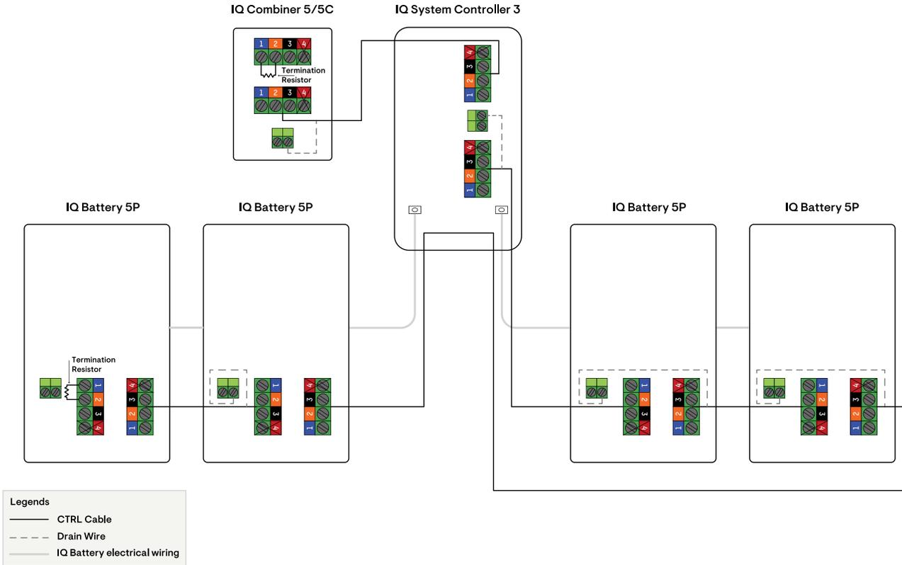
✓ **NOTE:** Total length of CTRL wiring across the system cannot exceed 250 feet to ensure the system operates as per specifications.
