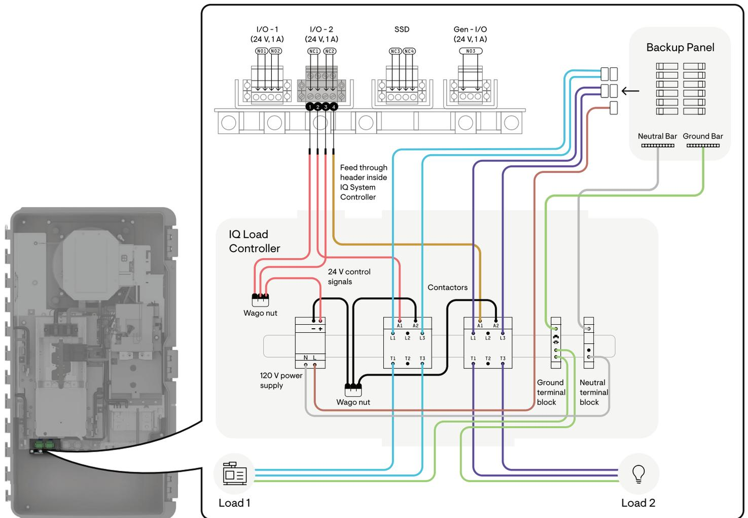
**NOTE:** Control lines to headers support 28 AWG and 16 AWG wire gauges.
