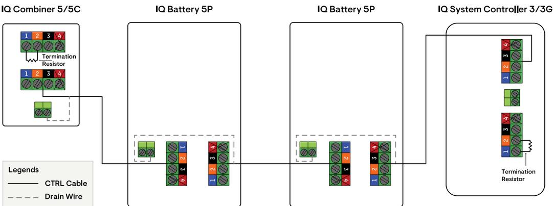
✓ **NOTE:** The total length of CTRL wiring across the system cannot exceed 250 feet to ensure the system operates as per specifications.
